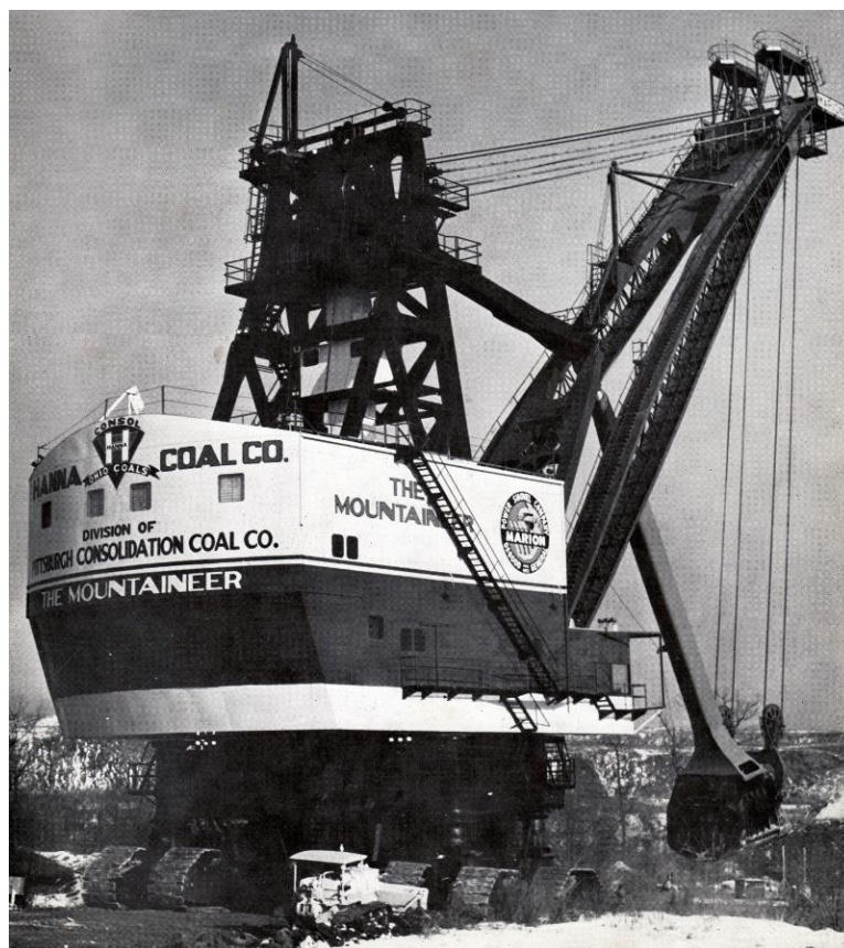
Obr. 43 Prvé mamutie dolovacie rýpadlo, Marion Model 5760 – The Mountaineer [50]
